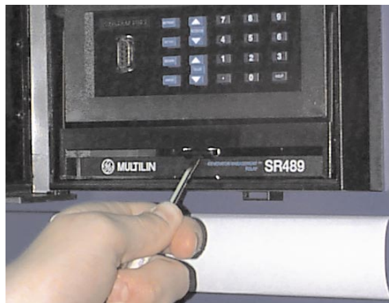
Figure 2–5: PRESS LATCH TO DISENGAGE HANDLE
